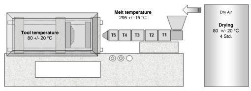
Typical filling pressure: Typical holding pressure: Typical holding time: 900 bar absolute +/- 25% 60 % of filling pressure 2 +/- 1 sec/mm wall thickness Back pressure: Typical cooling time: Average shrinkage: preferably low 2-3 sec/mm wall thickness 0,5 % flow / 0,85 % perp.
